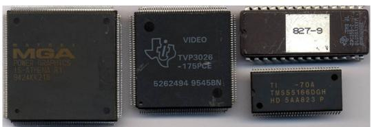
Core: IS ATHENA ?MHz 64bit Memory: 2MB (6MB max) VRAM ?MHz 64bit Year: 1994 Bus: PCI Made: 0,50 μm Links: stason.org infoworld Datasheet Price: \$599
