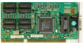
Core: TVGA9000i-3 ?MHz ?bit Memory: 1MB DRAM ?MHz 16bit Year: 1995 Bus: ISA 16bit Made: ? Links: none known
