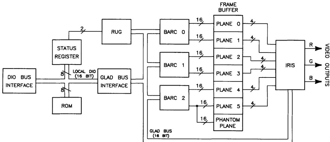
**Figure 3-10. Video Circuit Block Diagram**
