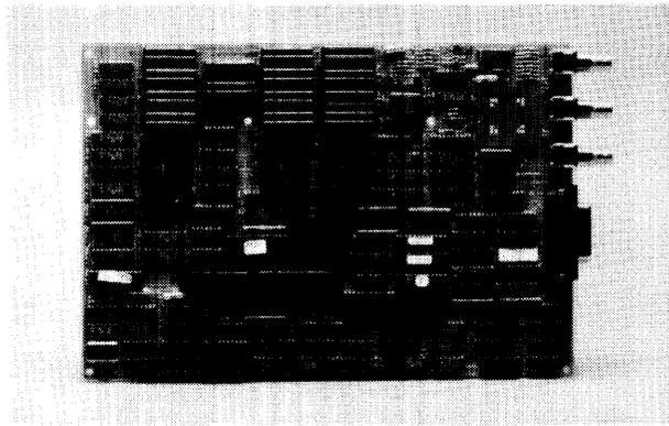
**Figure 3-9c. Video Board with Video and High-Speed HP-IB Circuits**
