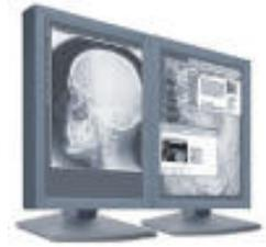
DuoView integrates a single display adapter capable of outputting to two monitors. Each output device can be configured through the S3Graphics Screen Goodies toolkit for its own independent refresh rate, resolution, and color depth. The Single Adapter Multi-Monitor DuoView implementation in UniChrome Pro allows different images to be displayed with independent timings, so a secondary monitor won't be limited to a laptop's 60Hz refresh rate.
