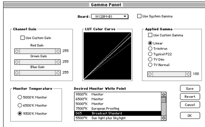
The color temperature of your monitor can be altered by selecting the monitor temperature setting (5000, 6500, 9300) that is closest to your monitor's factory setting and choosing the desired color temperature from the list.
