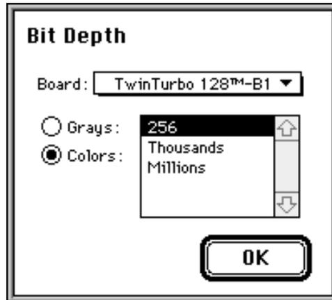
The color depth can be changed between 256 colors, Thousands (65,565) of colors, and Millions (16.7 M) of colors instantly via the Monitors Control Panel. Greyscale can be selected when using 256 colors mode. It is desirable to use the lowest colors possible for a particular application as the Twin Turbo-128 Display Adapter operates faster in reduced color depths. Refer to Table 3.1 for the available colors at a particular resolution.
