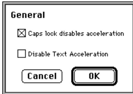
Graphics Acceleration on the Twin Turbo-128 can be disabled at any time by depressing the Caps-Lock key on the keyboard. This is useful for comparing the performance gains using Graphics Acceleration. To have the Caps-Lock key disable acceleration, check the box shown. Text caching can be disabled by checking the box shown.
