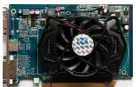
Core: Redwood XT 775MHz Shaders: 400 Memory: 512MB GDDR5 4000MHz 128bit Year: 2010 Bus: PCI-E 16x 2.0 Made: TSMC 40nm Taiwan Links: Legit OpenGL Price: \$99 / \$130 (1GB)
