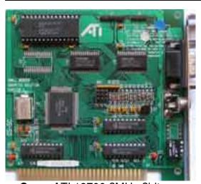
Core: ATI 18700 ?MHz ?bit Memory: 64kB ?MHz ?bit Year: 1988 Bus: ISA 8bit
