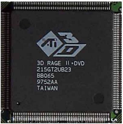
Core: ATI 3D Rage II+ DVD ?MHz ?bit Memory: 2/4MB SGR/EDO 67/60MHz ?bit
