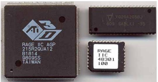
Core: ATI Rage IIC AGP ?MHz 64bit Memory: 4-8MB EDO / SDR / SGR 42 - 66MHz 64bit Year: 1998 Bus: AGP 1x Made: Taiwan Links: ProgrammerguideW95 SDKw95
