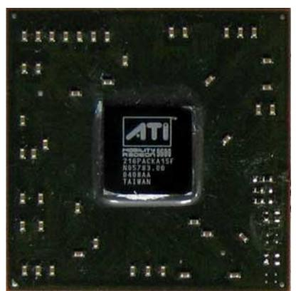
Core: RV350 325MHz ?bit Memory: 256MB DDR 400MHz ?bit Year: 2003 Bus: AGP 8x Made: TSMC 130nm Taiwan Links: Extremetech
