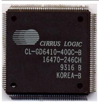
Core: CL-GD6410 25MHz ?bit Memory: 256kB DRAM ?MHz 16bit Year: 1992 Bus: integrated (ISA 16bit)
