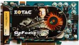
**Core:** G84 675MHz 32 shaders at 1458MHz **Memory:** 256MB GDDR3 2016MHz 128bit
