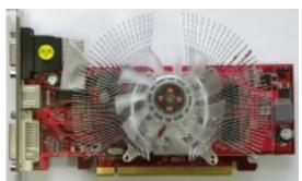
Core: RV610 700MHz 128bit Memory: 256MB GDDR3 1400MHz 64bit Year: 2007 Bus: PCI-E 16x Made: 65nm Unified Shaders:
