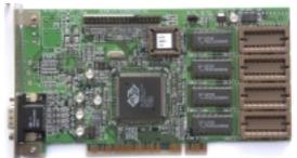
Core: ATI Rage II+DVD 75MHz 64bit Memory: 2/4MB EDO 60MHz ?bit Year: 1997 Bus: PCI Made: 350nm
