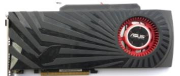
Core: Cypress XT 900MHz 256bit Memory: 2GB GDDR5 4800MHz 256bit Year: 2009 Bus: PCI-E 16x 2.1 Made: 40nm Transi stors: 2154 milion ROPs: 32 TMUs: 80 DirectX: 11 Unified shaders: 1600 (v 5.1) Memory bandwith: 153 ,6 GB/s Special: CrossFire Pixel fillrate: 28608 MPixel/s
