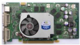
Core: NV41 350MHz 256bit Memory: 256MB DDR 600MHz 256bit Year: 2004 Bus:
