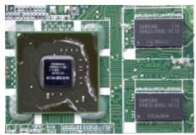
Core: N11M-GE2 625MHz 128bit Shader: 1530MHz Memory: 512MB GDDR3 1600MHz 64bit Year: 2010 Bus:
