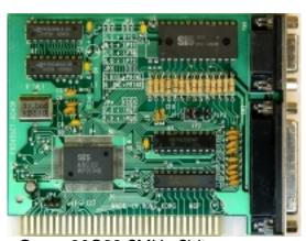
Core: 86C22 ?MHz ?bit Memory: 64kB ?MHz ?bit Year: 198x Bus: ISA 8bit Made: ? Links: none known
