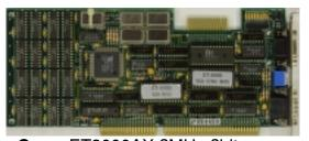
Core: ET3000AX ?MHz ?bit Memory: 512?kB ?MHz ?bit Year: 1987 Bus: ISA 16bit
