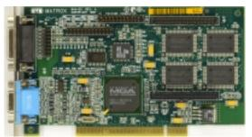
Core: MGA-1164SG-A (Cyclone) 66MHz 64bit Memory: 2/4MB(8MB max) SGR 99MHz 64bit
