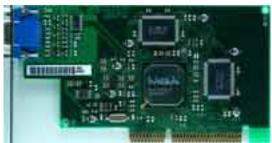
PRODUCTIVA **Core:** MGA-G100A-E (Twister) 41,40MHz 64bit **Memory:** 4/8MB SGRAM/SDR 62MHz 64bit **Year:** 1998 **Bus:** AGP1x
