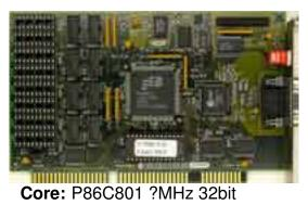
Core: P86C801 ?MHz 32bit Memory: 1MB DRAM ?MHz ?bit Year: 1992 Bus: ISA 16bit
