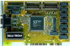
Core: 86C764-P ?MHz 64bit Memory: 1-2MB FPM/EDO ?MHz 32/64bit Year: 1994 Bus: PCI, VL-Bus Made: Taiwan Links: <u>Gbooks</u> info
