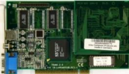
Core: 86C988 50MHz 64bit Memory: 4 (8 max) MB VRAM ?MHz 64bit (+ 2MB EDO RAM ?MHz - Elsa Winner 3000) Year: 1995 Bus: PCI
