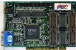
Core: 86C325 50/55MHz 64bit Memory: 2-4MB 1 cycle EDO 50/55MHz 64bit Year: 1996 Bus: PCI Made: Taiwan Links: Pdf Datasheet
