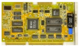
Core: WD90C11-LR ?MHz ?bit Memory: 512kB ?MHz ?bit Year: 1991 Bus: ISA 16bit Made: ? Links: none known
