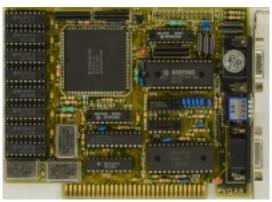
Core: PVGA1A-JK ?MHz ?bit Memory: 256kB ?MHz ?bit Year: 1988 Bus: ISA 8/16bit Made: ? Links: none known
