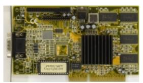
Core: Intel 740 66MHz 64bit Memory: 8MB SDR 100MHz 64bit Year: 1997 Bus: AGP 2x Made: 0,35μm, Intel Links: <u>Wikipedia</u> <u>Pdf</u>
