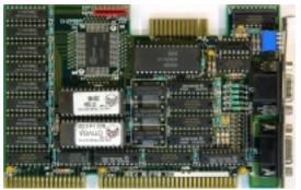
Core: UM587 ?MHz ?bit Memory: 512kB ?MHz ?bit Year: 1989 Bus: ISA 16bit Made: ? Links: Pdf
