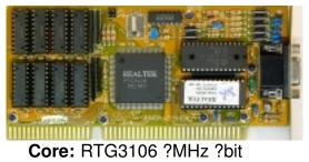
Core: RTG3106 ?MHz ?bit Memory: 512kB ?MHz ?bit Year: 1992 Bus: ISA 16bit Made: ? Links: none known
