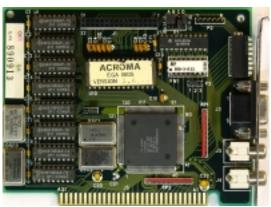
Core: VC-001 ?MHz ?bit Memory: 256kB ?MHz ?bit Year: 1987 Bus: ISA 8bit Made: West Germany, Japan Links: none known
