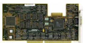
Core: Compaq 128084-004 ?MHz ?bit Memory: 1MB ?MHz ?bit Year: 1991 Bus: ISA 16bit/EISA Made: Japan Links: <u>Press</u> Price: \$599
