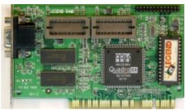
Core: ARK2000MI+ Quadro64 ?MHz 64bit Memory: 1-2MB EDO ?MHz ?bit Year: 1997 Bus: PCI Made: ? Links: ?
