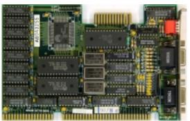
Core: OTI037C ?MHz ?bit Memory: 256kB ?MHz ?bit Year: 1988 Bus: ISA 8/16bit Made: ? Links: Pdf
