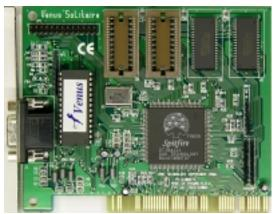
Core: OTI64111 Spitfire?MHz 64bit Memory: 1/2MB DRAM ?MHz ?bit Year: 1995 Bus: PCI Made: ? Links: Pdf Press
