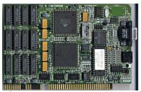
Core: 28800-6 & 38800-1 (Mach 8) ?MHz ?bit Memory: 1MB DRAM ?MHz ?bit Year: 1991 Bus: ISA 16bit
