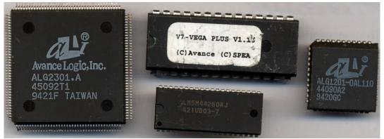
Core: ALG2301.A ?MHz ?bit Memory: 1MB ?MHz ?bit Year: 199? Bus: PCI Made: Taiwan Links: none known
