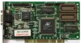
Core: ALG2302.A ?MHz ?bit Memory: 1MB (2MB max) ?MHz 32bit Year: 1995 Bus: PCI Made: Taiwan Links: info
