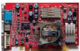
Core: RV380 500MHz ?bit Memory: 128MB DDR 700MHz 128bit Year: 2004 Bus: PCI-E 16x Made: TSMC 130nm Links: Guru3D Opengl
