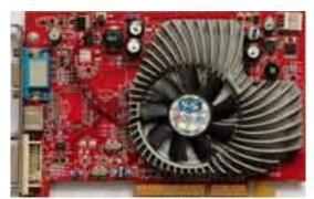
Core: RV530 500MHz 256bit Memory: 256MB DDR2 584MHz 128bit Year: 2005 Bus: AGP 8x / PCI-E 16x Made: TSMC 90nm Links: <u>Sapphire</u> <u>Tom's HW</u> <u>Legit</u> <u>OpenGL</u>
