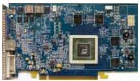
Core: R480 400MHz ?bit Memory: 256MB GDDR3 980MHz 256bit Year: 2005 Bus: PCI-E 16x Made: TSMC 130nm Taiwan Links: Tweaktown
