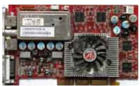
Core: R350 380MHz ?bit Memory: 128MB DDR 680MHz 256bit Year: 2003 Bus: AGP 8x Made: TSMC 150nm Taiwan Links: Hexus
