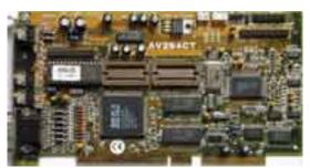
Core: ATI Mach 64CT ?MHz 64bit Memory: 1MB (2MB max) 50,272MHz ?bit Year: 1995 Bus: Asus Media Bus (PCI compactible) Made: Malta Links: <u>SDK</u>
