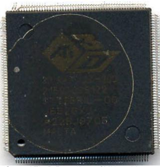
Core: ATI 3D Rage II-200 ?MHz 64bit Memory: ?MB ?MHz ?bit Year: 199? Bus: integrated in NB Made: Malta Links: none known
