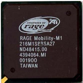
Core: ATI Rage Mobility M1 ?MHz ?bit Memory: 8MB integrated ?MHz ?bit Year: 1999 Bus: integrated Made: Taiwan Links: <u>Press</u> <u>Programmerguide</u>
