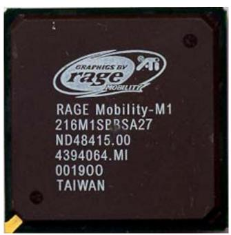
Core: ATI Rage Mobility M1 ?MHz ?bit Memory: 8MB integrated ?MHz ?bit
