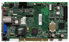
Core: ATI Rage XL ?MHz 64bit Memory: 8MB SDR ?MHz ?bit Year: 1999 Bus: PCI 32/64bit
