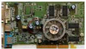
Core: RV350 391,5MHz ?bit Memory: 128MB DDR 445,5MHz 128bit Year: 2003 Bus: AGP 8x Made: TSMC 130nm Taiwan Links: <u>Wikipedia</u>
