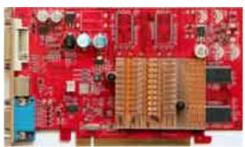
Core: RV370 324MHz ?bit Memory: 128MB DDR 392MHz 64bit Year: 2004 Bus: PCI-E 16x Made: TSMC 110nm Links: <u>MSI</u> <u>HW secrets</u> <u>Hexus</u> <u>OpenGL</u>
