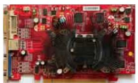
Core: RV515 594MHz ?bit Memory: 256MB DDR2 784MHz 128bit Year: 2005 Bus: PCI-E 16x Made: TSMC 90nm Links: MSI HW secrets Hexus OpenGL
