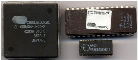
Core: CL-GD5434 108MHz 64bit Memory: 1MB (4MB max) FPM 50MHz 64bit Year: 1995 Bus: PCI Made: Korea/Taiwan/Japan Links: web archive pdf
